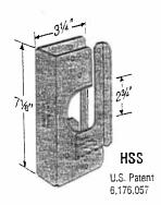
Heavy stud shoes provide tension load capacity as well as increased compression loads. Installs over pipe up to 2% outside diameter. See back for load information.
