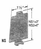
Prevents penetration of fasteners into electrical wires or plumbing pipe. Attach with 8d commons. 16 gauge to meet code.
