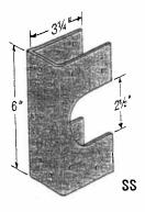
Stud shoes reinforce studs notched in construction. See back for load information. Available in sizes for 2x, 2-2x, 3-2x, and 3x studs. 16 gauge to meet code.
