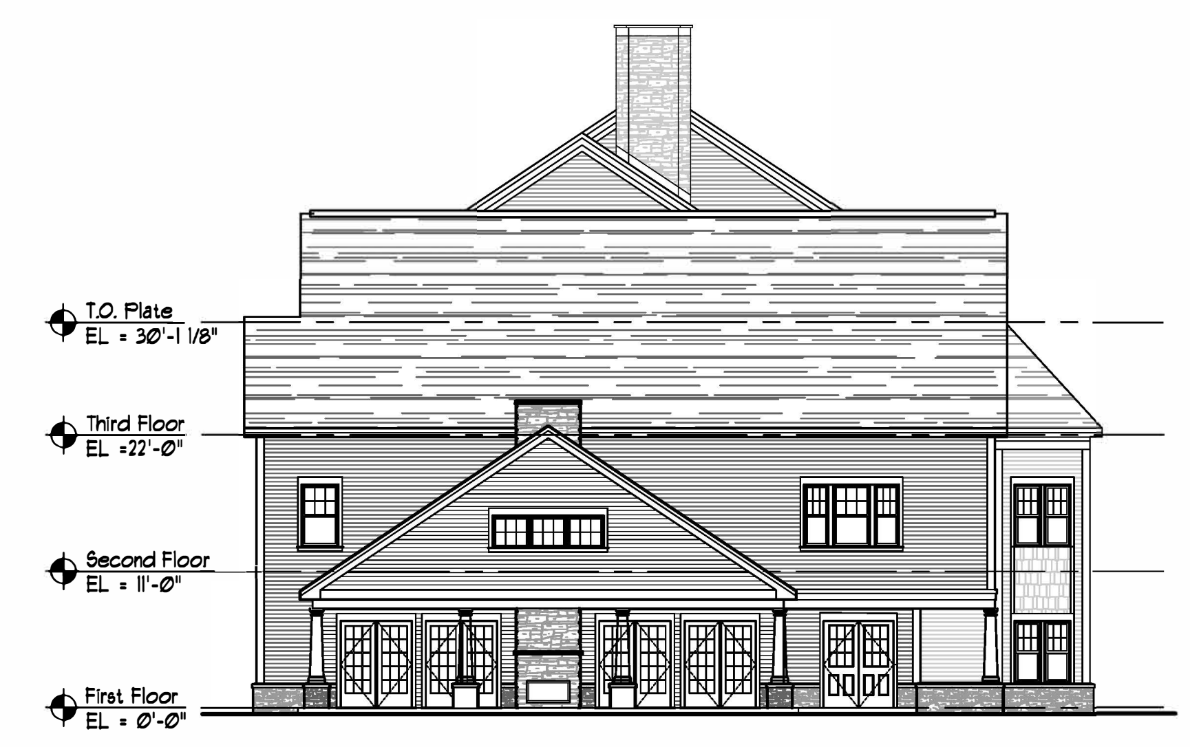
① SOUTH ELEVATION SCALE: 3/32"=1'-0"
